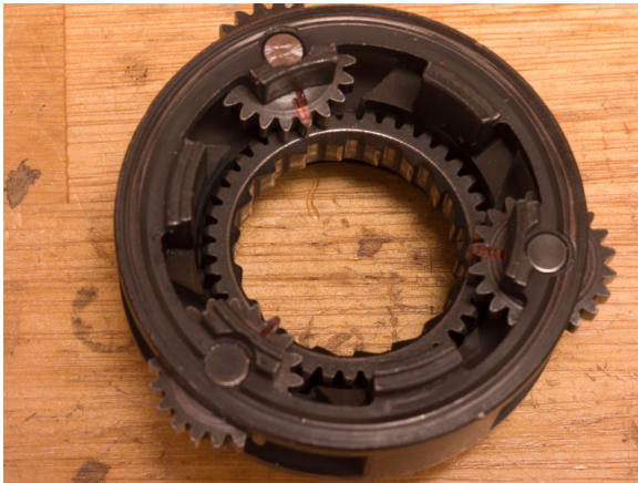
Figure 17. Gears placed correctly, with the markings pointing toward the center.
