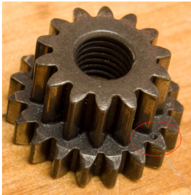
Figure 20. small gear. Note the alignment hole at the lower right.
