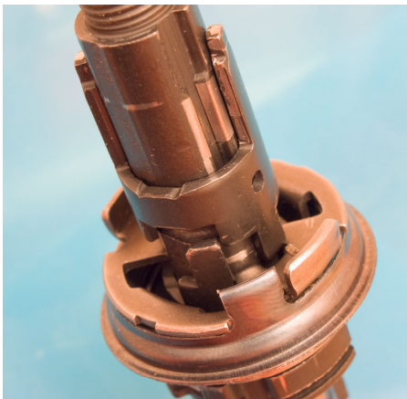
Figure 9. Test fitting and proper alignment of the shifter sleeve.
