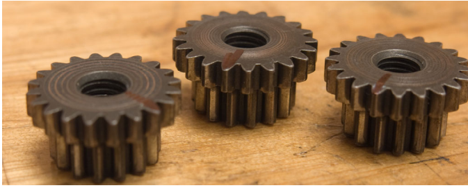
Figure 16. small gears marked (black line) where the small and big teeth line up.
