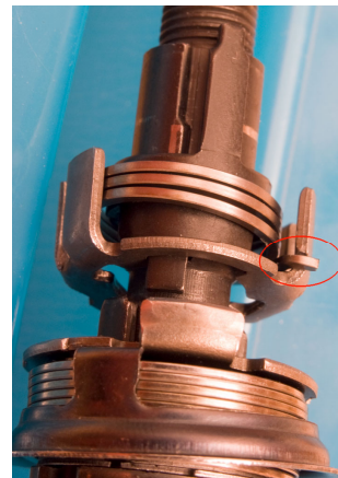
Figure 10. The small gear assembly mounted correctly and ready to slide into the return spring assembly.
