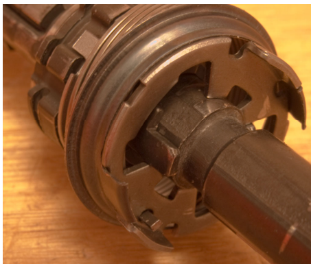
Figure 7. Return spring loaded and held by the return spring loader ring.
